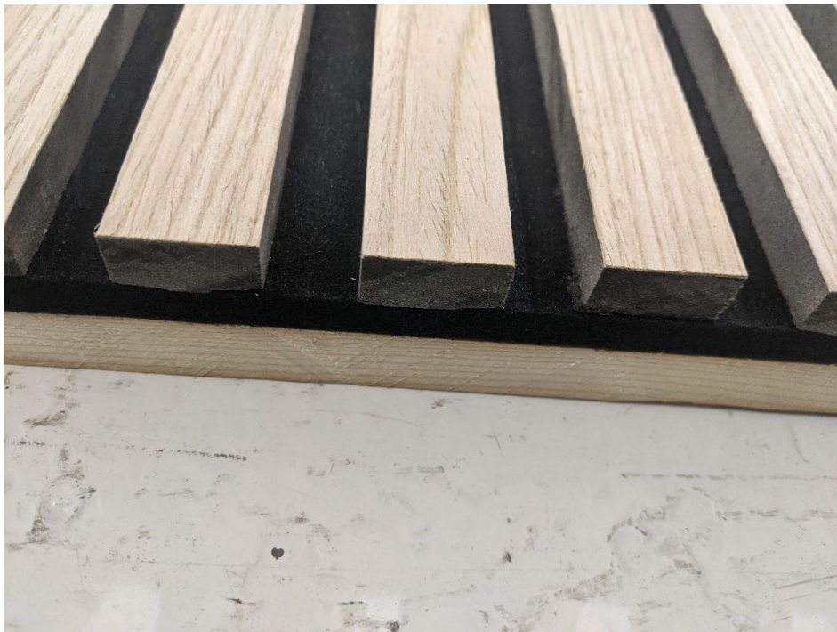
Figure 4 – Detail of specimen materials, as installed over furring strips
