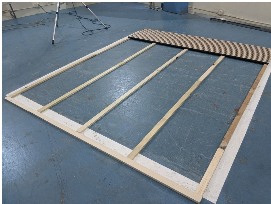
Figure 2 – Specimen partially installed over spaced furring strips
