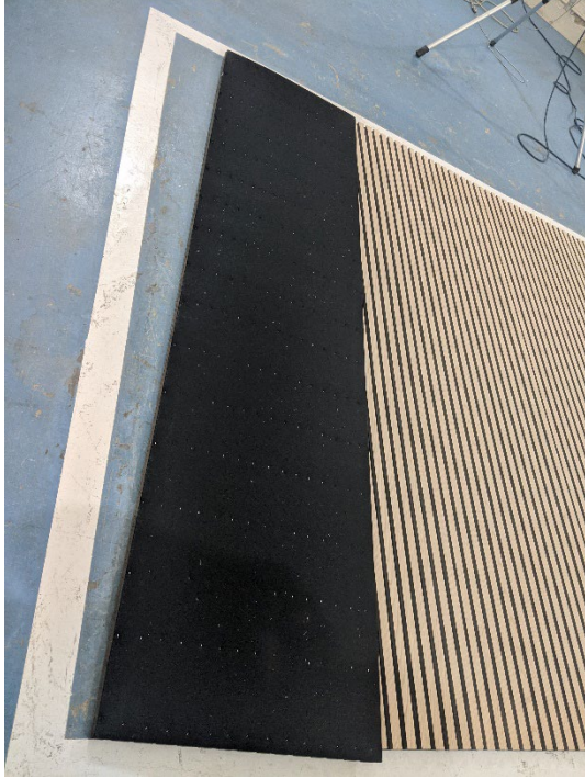
Figure 3 – Individual specimen panel, face mated to horizontal test surface
