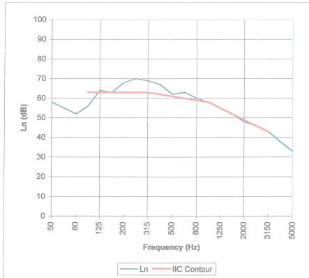
L<sub>n</sub> = Normalized Sound Pressure Level, dB
