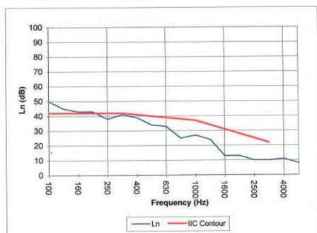
Due to high insulating value of specimen, background levels limit results at these frequencies.
