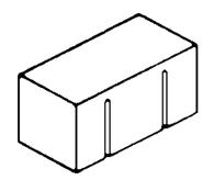
Open top, non-slotted cavities for reinforcing bars and grout
