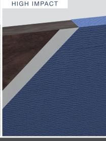
The BioCore Wall Panels are offered in two styles - Standard & High Impact. The Standard Panel's core consists of a 6-7 lb. density rigid fiberglass board. The High Impact Panel adds an additional 1/8" thick high density layer, which is ideal in higher traffic areas or when there is a desire to have a high level of tackability from the panel. BioCore Panels are offered in a wide variety of fabrics leaving a straight, flat wrinkle-free surface with tailored corners.
