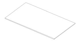
3. Use the putty knife to place the carpet adhesive to one TETRIX™ at a time. Working on one TETRIX™ at a time, apply a liberal amount of adhesive to the back of the panel utilizing the adhesive manufacturers best practices.
