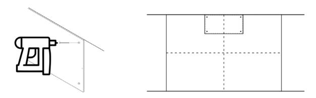
6. Use a box cutter and metal ruler to make cuts to fit the wall.
