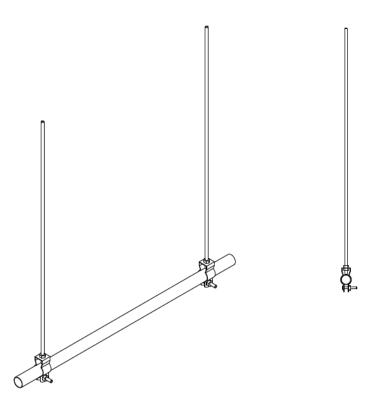
2. Make 1/4" drill for threaded rod assembly.
