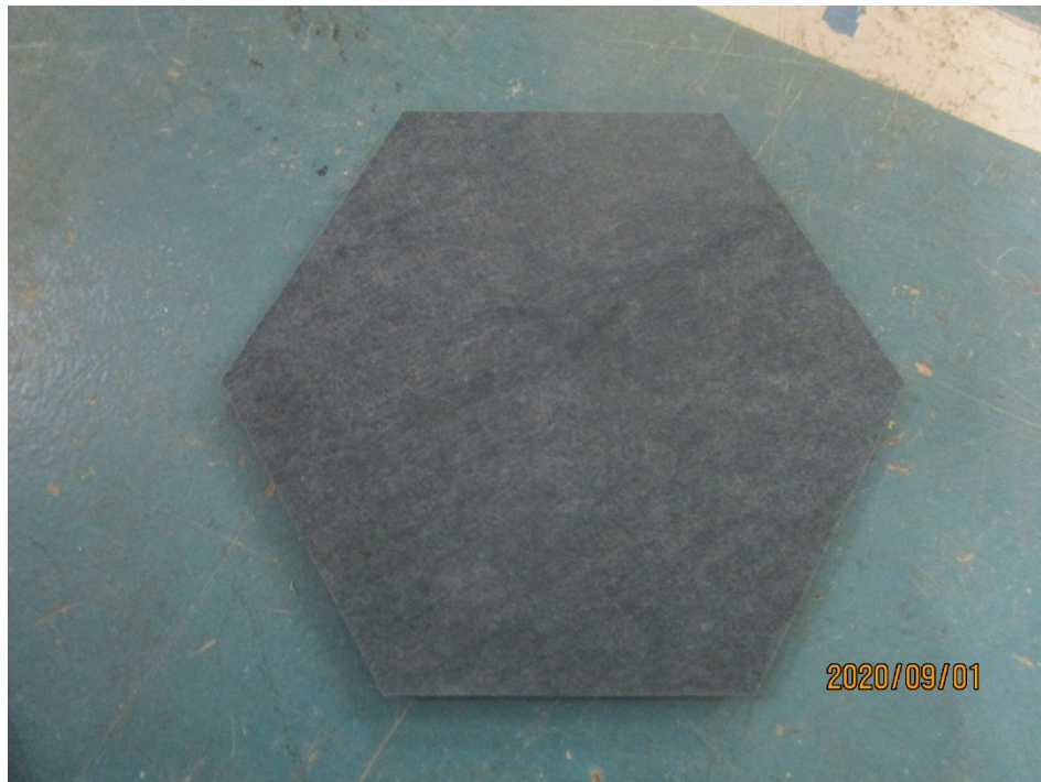
Figure 3 – Individual panel specimen, face mated to horizontal test surface
