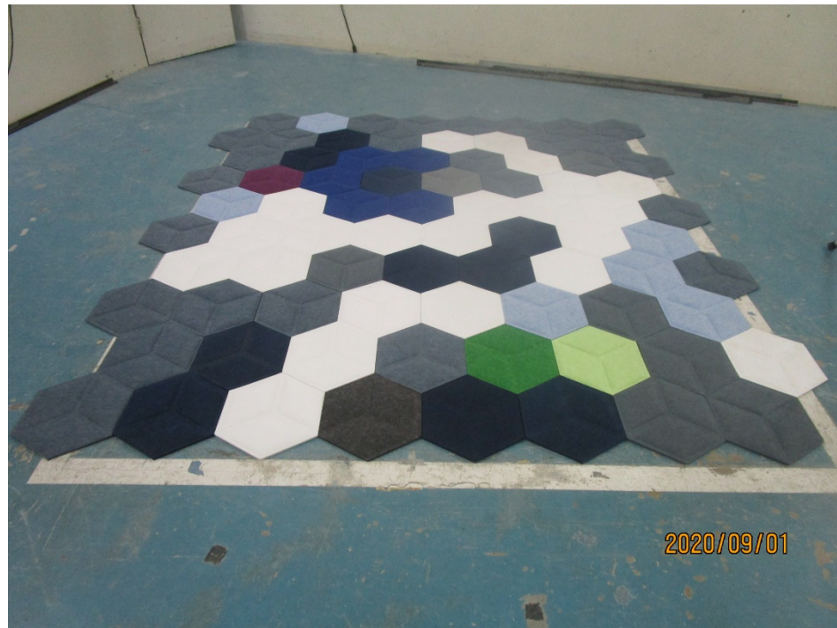
Figure 1 – Specimen mounted in test chamber
