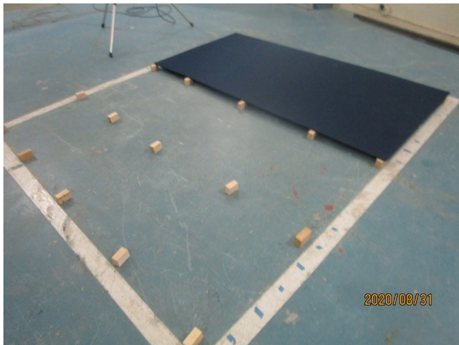
Figure 2 – Specimen partially installed, spacer array
