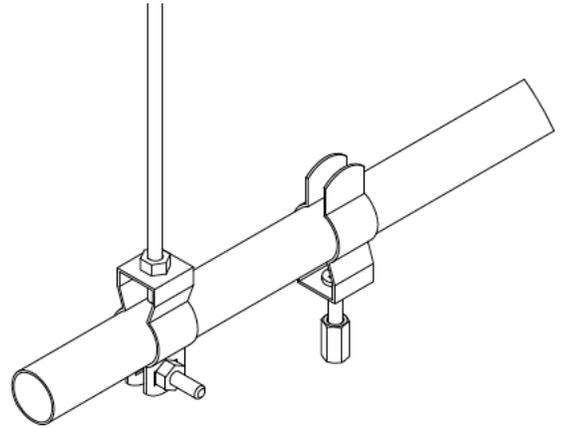
4. Insert the threaded rod to the coupling nut.
