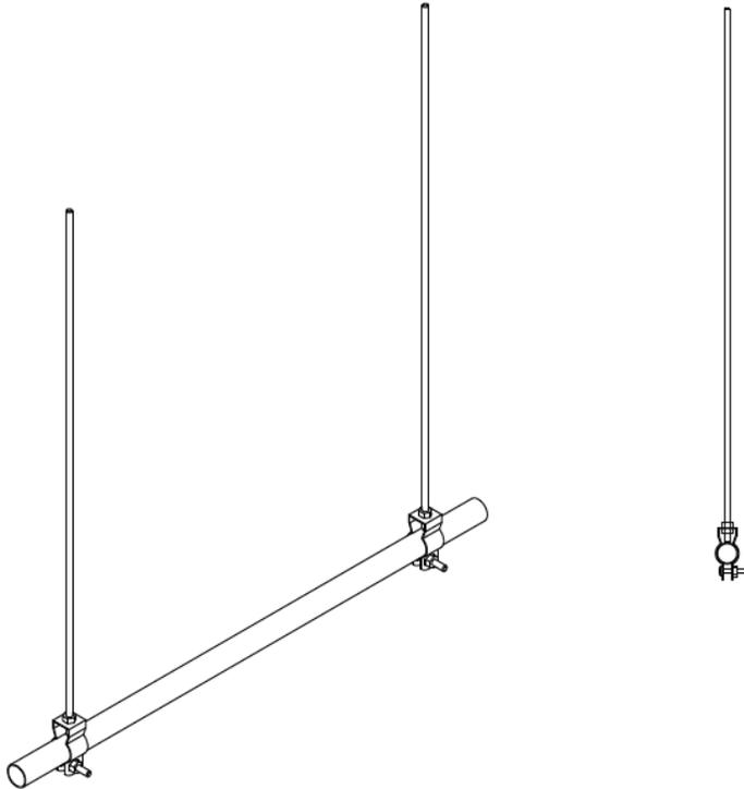
2. Make 1/4" drill for threaded rod assembly.
