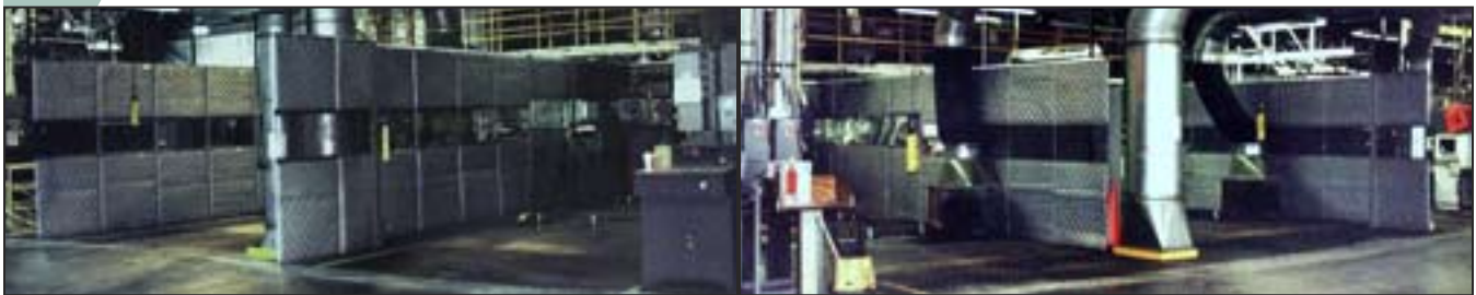
Sound Seal BSC-25 Acoustical Curtain Panels with full width clear vinyl view windows form a three-bay acoustical curtain enclosure at a Ford Motor Company plant.
